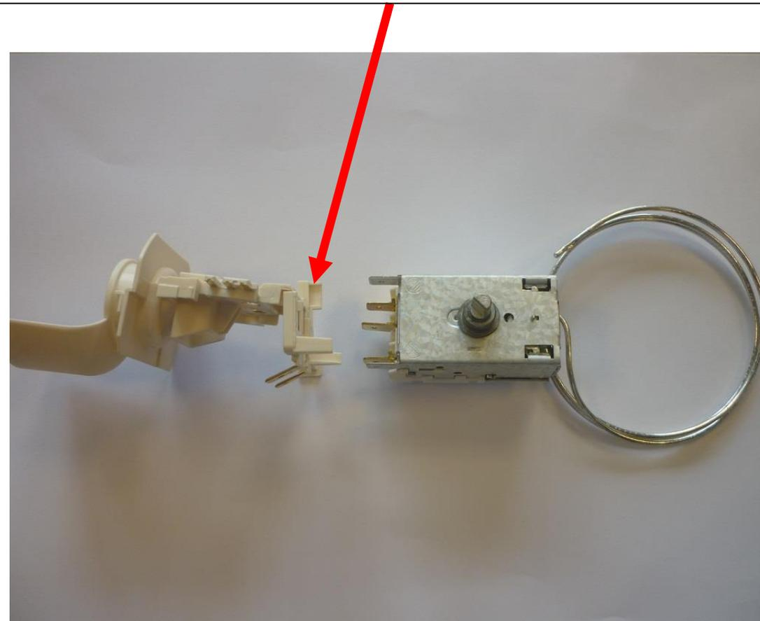
Bend the rear part of the lamp holder with 90 degrees, so that it fits the plug connections of the thermostat!
