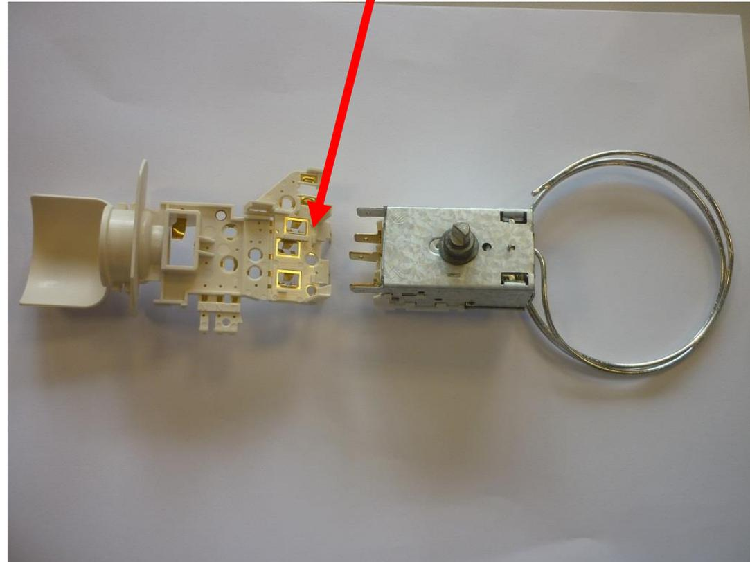
Bend the rear side of the lamp holder with 90 degrees, so that it fits the plug connections of the thermostat!
